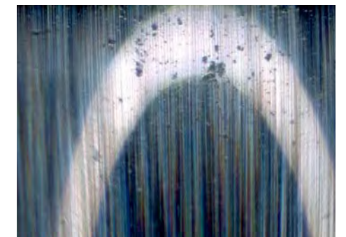
Indentations in raceway caused by particles
